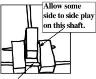
This part will need to be removed when the glue is dry. A blob of glue can be added to the ends for extra strength. Allow a little play at the crank follower end so that it can clear the lower supports.
